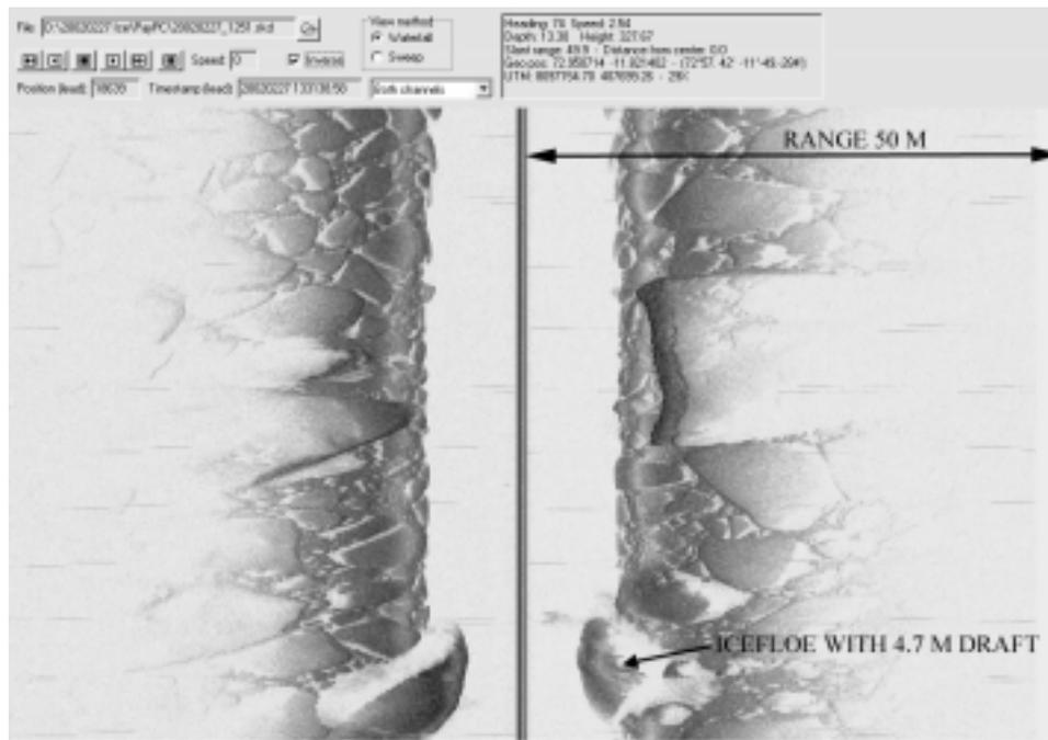
SIDESCAN IMAGE NOT CORRECTED FOR SLANT RANGE
