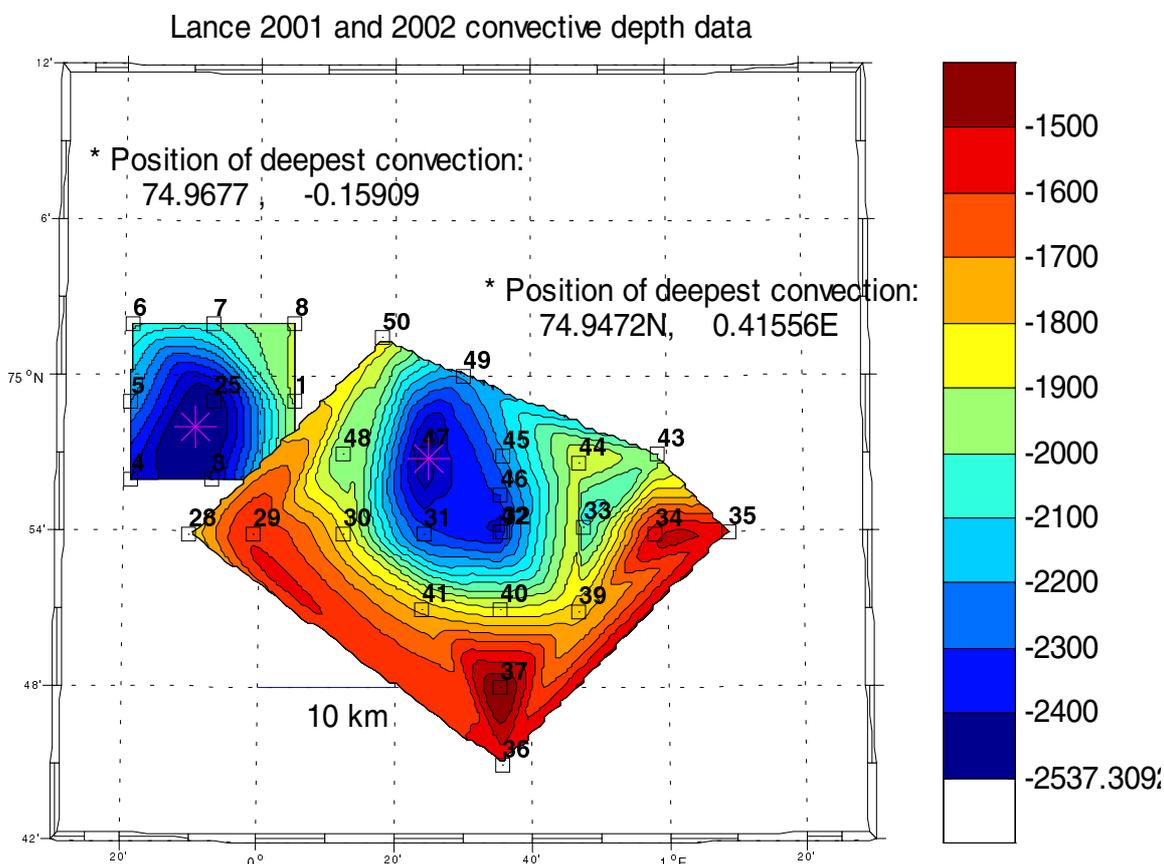
Convection depths of the chimney. Last year's survey (larger picture), this survey (smaller picture).
